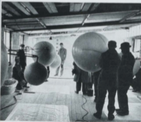
Production line for rubber balloons. Exact amount of hydrogen is measured by the balancing on arm on the filling device, an invention of Czech member of Free Europe Press. Workers seal filled balloons with leaflets inside.
